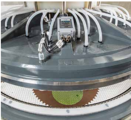
The temperature sensor measures the temperature at the inner and outer diameter during the process and visualizes it on the HMI
