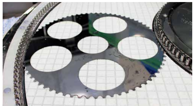
A carrier guide ensures safe processes even with thin workpieces
